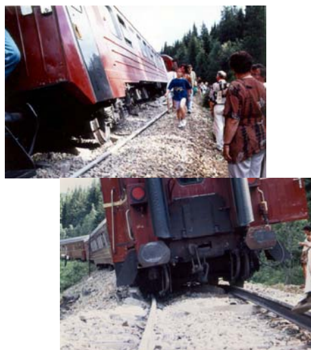
Fig.32 Typical minor railcar derailment due to a bearing capacity failure caused by a loss of soil suction
